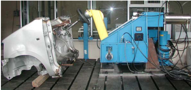
Steering Column Displacement against Front Collision
