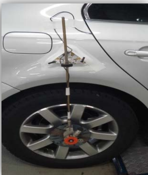
Wheel Pulse Transducer (WPT)
