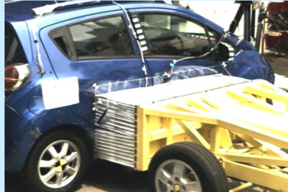
Side Impact Test
