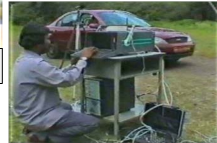
Pass-by Noise Test
