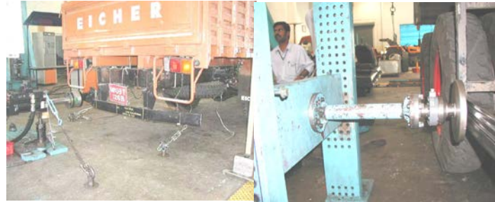
Rear and Lateral Under Run Protection Devices against Front Collision
