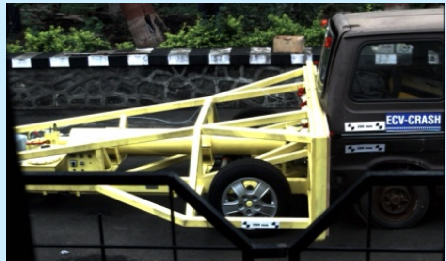
Rear end Impact Test
