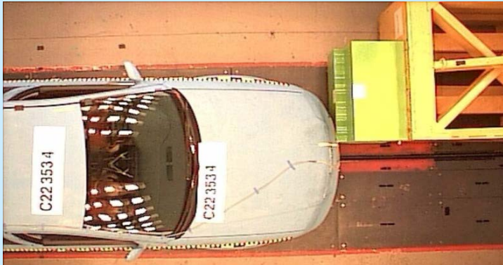
Offset Frontal Test
