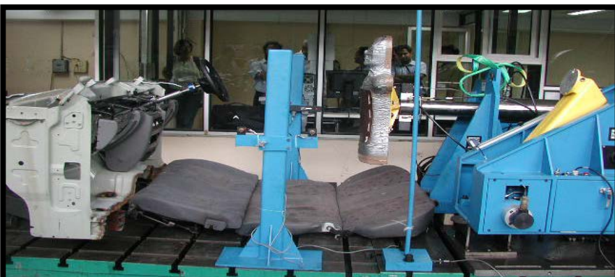
Velocity Generator for Body Block Impact Test and Head Form Impact Test
