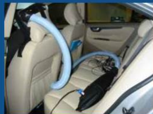
Reciprocal method using volume velocity source
