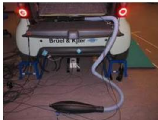
Measurement of acoustical path sensitivities
